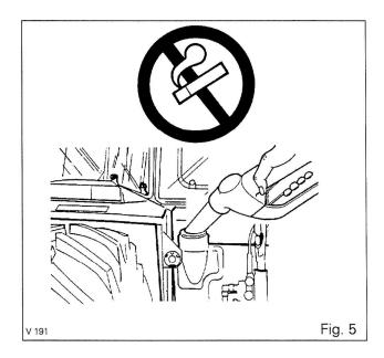
CAUTION: Access to fuel filler by means of climbing onto non-rigid linkage elements is not permissible.
