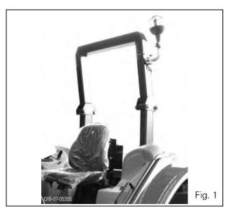
IMPORTANT: The Roll Over Protection Structure (ROPS) only offers partial protection against loads falling on the operator's seat, and additional protection can only be obtained by using implements designed to prevent loads from falling on the operator's seat.
