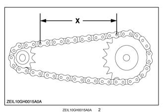
**Measurement of Chain For Wear Elongation**
