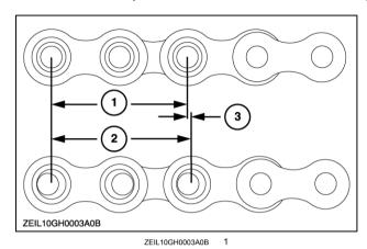
Chains do not "stretch" - material is removed from pin and bushing.
