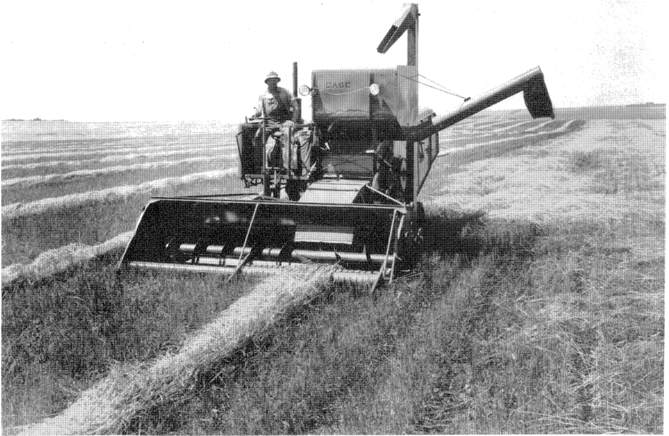
Figure 5. Field View of Model SP-12 Self-Propelled Combine Equipped with Pick Up Attachment
