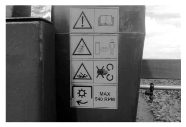
The following safety signs are placed on the machine and care should be taken in respect of the dangers they are warning against:
