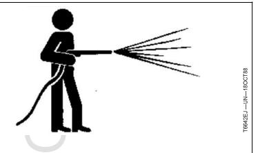
If a cleaning agent is used, the agent must be the correct concentration. Do not allow cleaning agent to dry on machine, promptly rinse from top to bottom. Your John Deere dealer has cleaners which are compatible with your equipment and which are recommended to remove protective shipping coatings.
