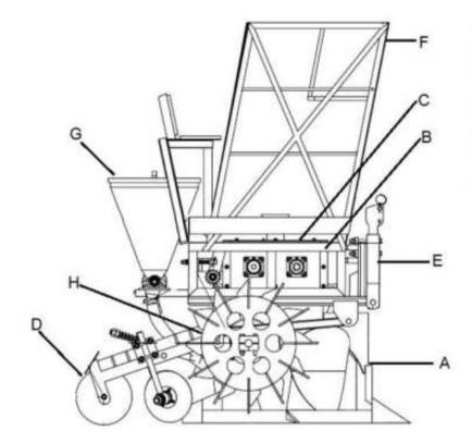
A = Main Frame B = Frame Support C = Cutting Box D = Roller E = Holder Linkage F = Basket G = Fertilizer Tank H = Wheels
