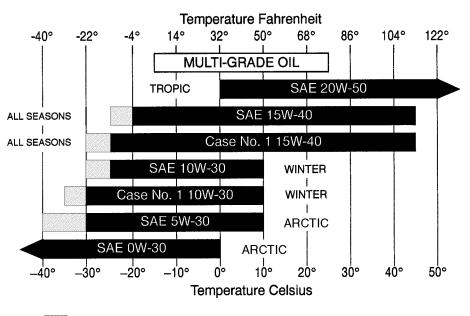
Indicates use of an engine oil heater or a jacket water heater is required.
