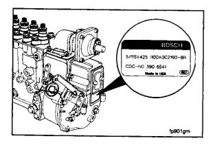
The Cummins part number for the fuel pump - governor combination is located on the governor dataplate.
