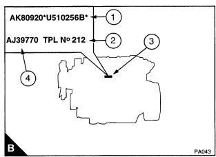
If a short engine is installed two engine serial numbers and a TPL number on the engine serial number plate (B3), examples are shown above.
