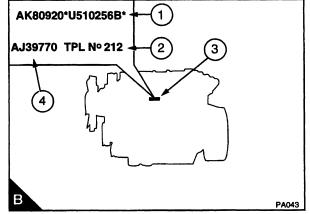
If a short engine is installed two engine serial numbers and a TPL number on the engine serial number plate (B3), examples are shown above.
