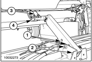
5. Start the tractor, raise the arms up to the maximum raised position and engage the header lock by pulling rearward on the handle. The header lock, 1, is located on the left front corner of the windrower. The handle is shown here in the locked position.
