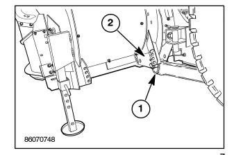
3. Remove the pin holding the header tilt cylinder in the storage position and connect it to the header using a clevis pin. On the RD182 header the cylinder only has one hole to connect to on the header. When the header tilt channel is installed in the rearward holes, 1, this provides a cutting range of 1-1/2 inch to 3 inch. When installed in the forward holes, 2, the cutting range is 1 inch to 2-1/4 inch. The forward holes on the tilt channel should be used for most crops.
