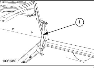
The right side shield can be lifted by releasing two rubber straps, 1, on the front and rear of the shield, and pivoting the shield upward. Lift the shield part way and remove the latch rod, 2, from the slot in the shield. Raise the shield fully and hook the rod into the slot in the top of the shield to support the shield.
