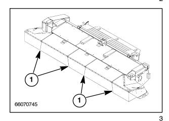
When raised, the front shields are held in place by a lever, 1. The lever automatically springs into the lock as the shield is raised. To lower the shield, release the lever by pushing it to the side.
