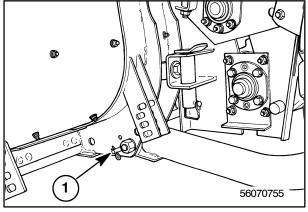
7. Disengage the header lift lock as shown.
