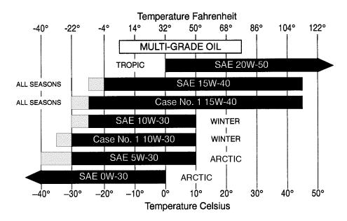
Indicates use of an engine oil heater or a jacket water heater is required.
