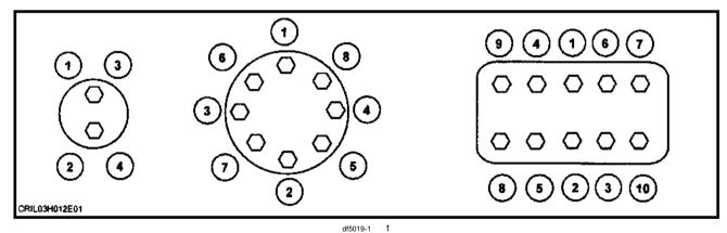
NOTE: Shown above is the suggested initial torque tightening sequences for general applications, tighten in sequence from item 1 through to the last item of hardware.
