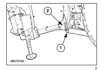
3. Remove the pin holding the header tilt cylinder in the storage position and connect it to the header using a clevis pin. On the RDX181 header the cylinder only has one hole to connect to on the header. When the header tilt channel is installed in the rearward holes, 1, this provides a cutting range of 1-1/2" to 3". When installed in the forward holes, 2, the cutting range is 1" to 2-"1/4. The forward holes on the tilt channel should be used for most crops.
