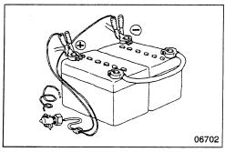
To apply voltage for testing, check that the positive and negative cables are connected properly, then increase voltage gradually from 0 volt. Do not apply voltage higher than the specified value.
