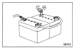
Before carrying out maintenance work on the electric system, disconnect the negative terminals of the batteries.
