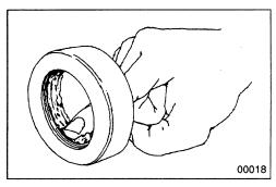
Apply the specified oil or grease to U-packings, oil seals, dust seals and bearings during assembly.
