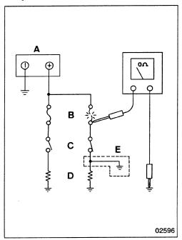
Remove fuse **B** and measure resistance between the loaded side of the fuse and ground.
