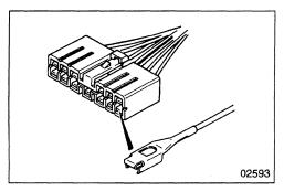
Check for a decrease in contact pressure between the male and female terminals.
