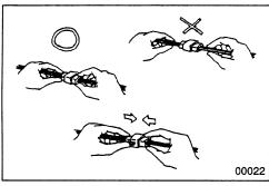
Pull the connector, and not the harness lead, to separate connectors.
