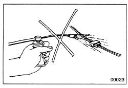
When washing the vehicle, cover the electric system parts and instruments with waterproof material beforehand (Cover with vinyl sheet or the like). Keep water away from harness wire connectors and sensors.
