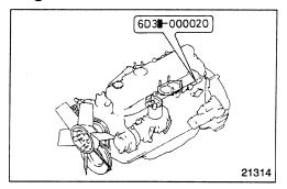
The engine number is punch-marked on the shown location.
