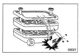
Take care when handling sensors, relays, etc. which are vulnerable to shock and heat.
