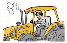
When the tractor is operated under full or partial load, the operator is exposed to continuous or intermittent level noise above 85 dB. (A), measured according to the procedure in the ABNT NBR 9999 standard.
