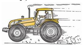
Adapt the speed of the tractor according to the ground conditions, the visibility conditions and the load to be transported. Avoid abrupt stops or sudden increases in the speed of operation, as well as sharp turns at high speed. This can cause the load or the tractor to tip over.
