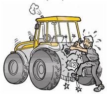
Keep away from components in motion, especially the engine and the PTO. When the PTO shaft is not in use, keep the cover in place.
