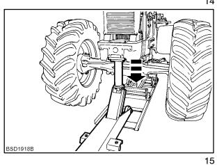
8. Disconnect and remove front wheel drive shaft universal joint.
