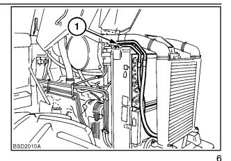
6. Withdraw condensor from front of radiator and place in a safe place on side of engine.
