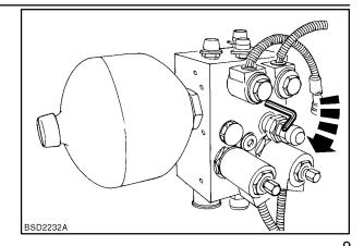
2. Disconnect the pipes to the front axle suspension cylinders.
