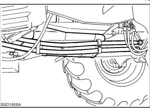
4. Remove the rear pivot block bolts.
