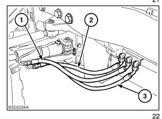
Inspect the harness connections between the engine and front support and disconnect where necessary to enable the front support and axle to be separated from the engine.
