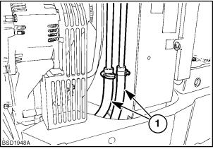
5. Remove clips (1) securing air conditioning condensor tubes to side of radiator.
