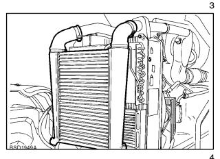
4. Disconnect transmission oil cooler hoses (1) and drain oil into clean container.
