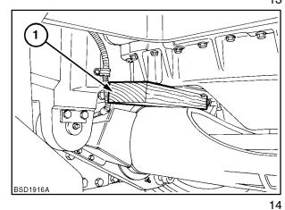
7. In a controlled manner lower the front of the tractor to the ground. The lowering action will cause the suspension arm pivot block to separate from the transmission casing.
