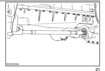
4. Disconnect power steering hoses (1) and (2) on each side of the tractor.
