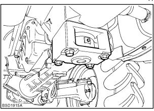
5. Position trolley jack beneath front support and raise front of tractor.
