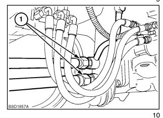
3. Remove suspension pipes and guard.
