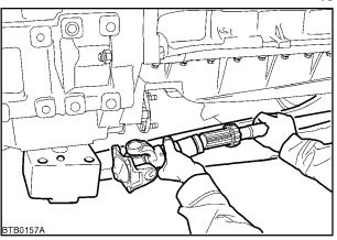
\_\_ 16 9. Remove engine side rails
