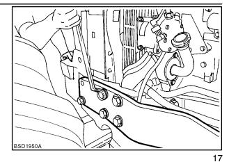
10. Disconnect the 2 steering tubes and differential lock tube from the right hand side.
