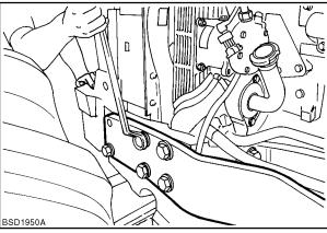
2. Remove front wheel drive shaft guard, if fitted.
