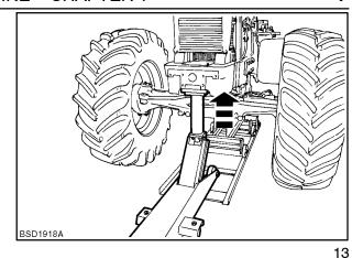
6. Position a suitable piece of strong timber between oil pan and suspension arm.
