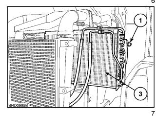
7. Drain the cooling system fluid into a clean container and disconnect the radiator hoses. Disconnection of the radiator lower hose provides a suitable drain point. Place a large clean tray under the vehicle to capture the fluid for future use.
