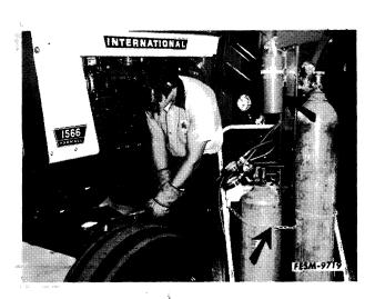
9. When using an acetylene torch always wear welding goggles and gloves. Keep a "charged" fire extinguisher within reach. Be sure the acetylene and oxygen tanks are separated by a metal shield and are chained to the cart. Do not weld or heat areas near fuel tanks or fuel lines and utilize proper shielding around hydraulic lines.
