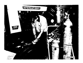
10. When using an acetylene torch always wear welding goggles and gloves. Keep a "charged" fire extinguisher within reach. Be sure the acetylene and oxygen tanks are separated by a metal shield and are chained to the cart. Do not weld or heat areas near fuel tanks or fuel lines and utilize proper shielding around hydraulic lines.
