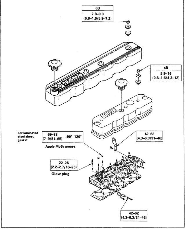
Mos2..... Molybdenum disulfide paste.
