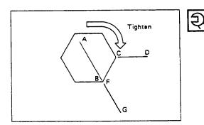
Draw another line (C-D) on the face of each of the parts to be clamped. This line should be an extension of the line [A-B].
