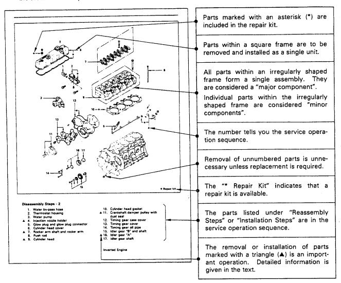
6. Each service operation section in this Workshop Manual begins with an exploded view of the applicable area. A brief explanation of the notation used follows.
