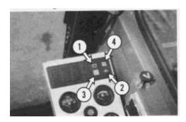
**Alternator (1.)** - This light monitors the charging system. It should light up when the engine OFF-ON-START key is turned to ON. If the light does not go off while the engine is running, the batteries are not being charged. The machine can be operated until repairs can be made. However, if the electrical accessories are used, the batteries will discharge rapidly.
