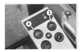
Fuel Level (3.) - Indicates the amount of diesel fuel in the fuel tank.
