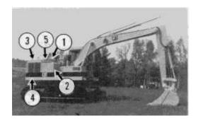
Engine (1), fuel tank (2), radiator (3), battery (4) and key disconnect switch (5).
