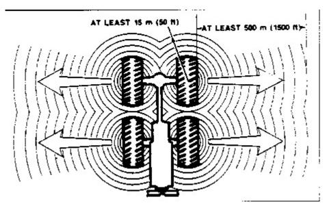
Do not approach a tire closer than the outside of the area represented by the shaded area in the above drawing.
