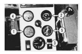
**Service Hour Meter (1.)** - Indicates the total number of hours the engine has operated. Use it to determine service intervals.
