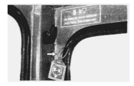
To remove rear window, pull ring and push out.
