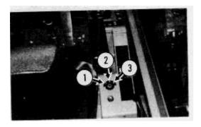
**OFF (1)** - No power to most electrical circuits in the cab. The cab lights, panel lights, tail lights and the fuel gauge light are operational even with the switch in the OFF position.
