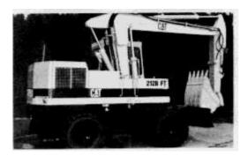
This machine is equipped with a 3114 diesel engine.
