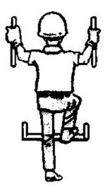
\* Face the machine when mounting and dismounting.
