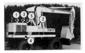
Engine (1), fuel tank (2), radiator (3), battery (4) and key disconnect switch (5).
