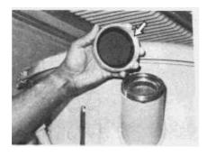
Remove the hydraulic tank filler cap only after the engine has been stopped and the filler cap is cool enough to remove with your bare hand.
