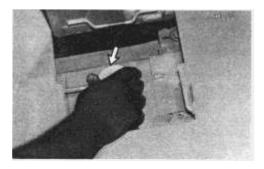
Check the coolant level only after the engine has been stopped and the filler cap is cool enough to remove with your bare hand.
