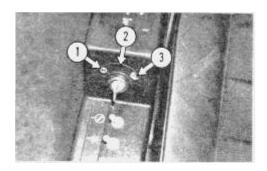
**OFF** (1.) - Turn the key to OFF before trying to restart engine after shutoff.
