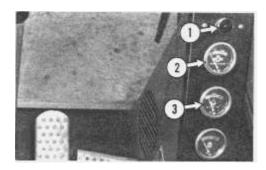
**Master Fault Light Indicator (1.)** - Flashes to alert the operator to take immediate action to prevent machine damage. The flasher operates if engine oil pressure is too low, or if engine coolant temperature is too high.
