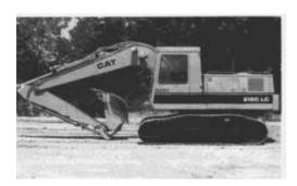
This machine is equipped with a direct-injection 3304 turbocharged engine. It has hydrostatic drive, variable flow hydraulics and spring applied/hydraulically released brakes.
