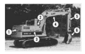
Engine (1), fuel tank (2), hydraulic tank (3), boom (4), stick (5) and bucket (6).
