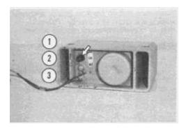
A switch at the rear of the alarm adjusts the sound level.
