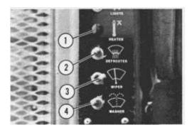
**1. Heater Switch -** Center the switch for low heater fan speed. Move the switch to the right for high fan speed. Move the switch to the left to turn the fan off.
