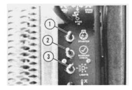
**1. Start Switch -** To crank the engine, pull up on the switch and move it to the right. If equipped with electric engine shutoff, move the switch to the left to stop the engine.
