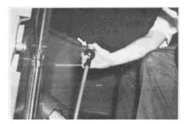
To stop the alarm when it is not needed, press the button, at the top of the steering control.
