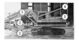
Use steps (1), (2) and (3) and grab irons (4) and (5) when entering or leaving the operator's compartment.
