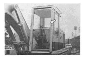
Use the front windshield as an emergency exit if the door is blocked.
