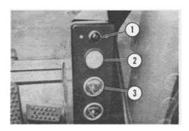
**Malfunction Warning Flasher (1.)** - Flashes to warn the operator to take immediate action to prevent machine damage. The flasher operates if engine oil pressure is too low, or if engine coolant temperature is too high.
