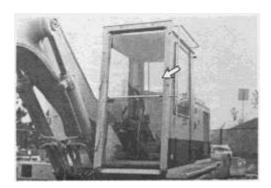
Use the front windshield as an emergency exit if the door is blocked.
