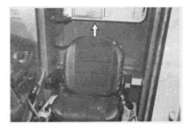
To adjust the seat back tilt, lift the back and tilt it to one of 3 positions. Release the back.
