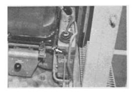
To permit moving the seat forward or rearward, push the lever, at the left side of the seat, toward the operator.
