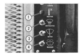
**1. Heater Switch -** Center the switch for low heater fan speed. Move the switch to the right for high fan speed. Move the switch to the left to turn the fan off.
