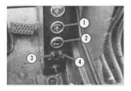
Hydraulic Oil Temperature (1.) - The gauge should register in the green range during operation.
