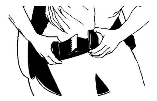
**2.** To remove the slack in the outer loop, rotate the buckle to free the lock bar. This permits the belt to move through the buckle.
