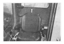
To adjust the seat back tilt, lift the back and tilt it to one of 3 positions. Release the back.
