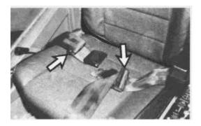
**2.** Inspect the adjusters for wear, damage and correct operation. Replace the belt if the adjusters are damaged or worn.
