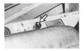
Lighter Push down the knob. The lighter moves up when it is ready for use.
