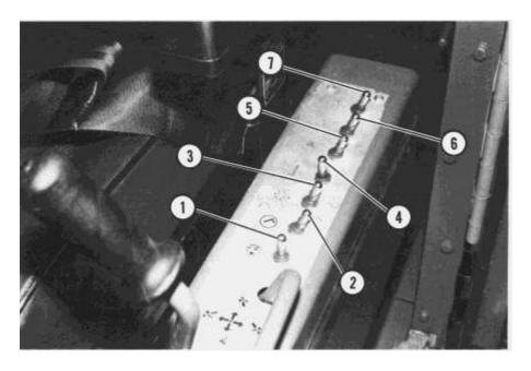
Start Switch (1) Pull the switch up and move it to the right to crank the engine.
