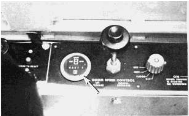
Electric Service Meter
