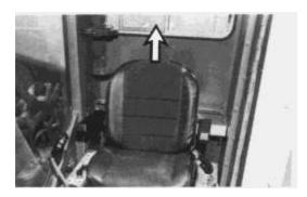
To adjust seat back tilt, lift the back and tilt to one of 3 positions. Release the back.
