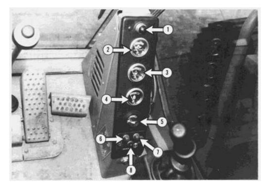
**Master Warning Light (Red) (1)** Flashes to warn the operator of a machine malfunction. It operates if engine coolant temperature is high, engine oil pressure is low or if the hydraulic oil level is low.
