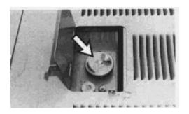
Remove the cooling system filler cap slowly to relieve pressure.
