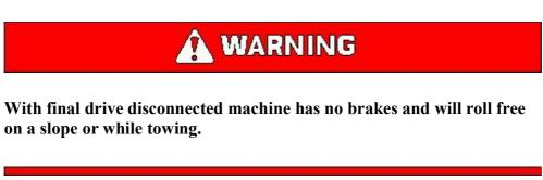
When final drive is disconnected always block both tracks.
