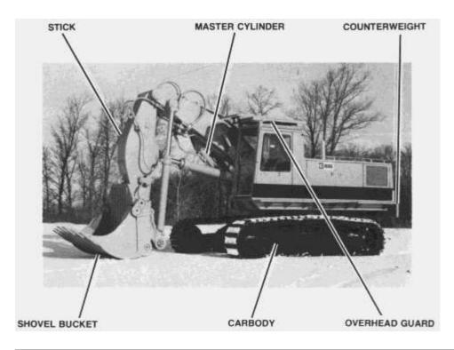
《Product: EXCAVATOR Model: 235 EXCAVATOR 81X Configuration: 235 EXCAVATOR 81X00404-UP (MACHINE) POWERED BY 3306 ENGINE
