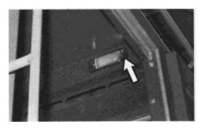
Interior Light Switch Move the switch to turn the cab inside light on or off.
