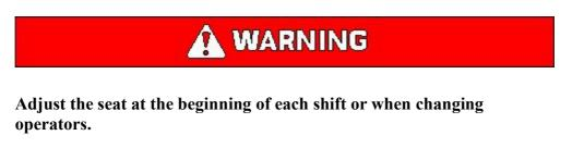
Adjust the seat to allow full travel of the pedals when the operator is seated against the seat back.
