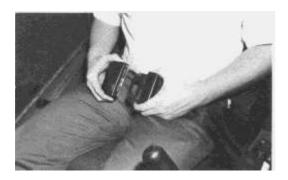
**5.** Fasten the buckle. Pull the loose ends of the belt to remove the slack. The belt should be snug but comfortable.
