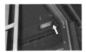
**Interior Light Switch** Move the switch to turn the cab inside light on or off.
