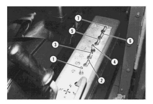
**Start Switch (1)** Pull the switch up and move it to the right to crank the engine.
