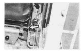
Push the lever to the right to permit moving the seat forward or backward.
