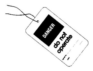
Do not start the engine or move any of the controls if there is a "DO NOT OPERATE" or similar warning tag attached to the start switch or controls.
