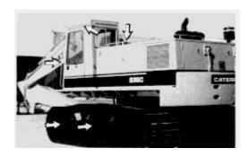
Mount and dismount the machine only where steps and/or handholds are provided.
