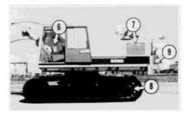
Operator's compartment (6), radiator (7), final drives (8), and counterweight (9).
