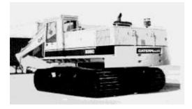
This machine is equipped with a direct-injection 3306 turbocharged and aftercooled engine. It has hydrostatic drive, variable flow hydraulics and spring applied/hydraulically released brakes.
