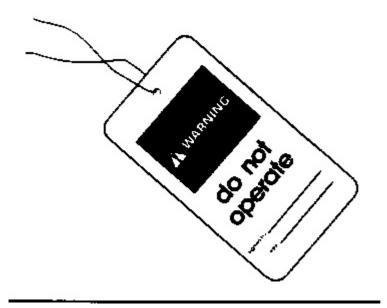
Attach a Do Not Operate, SEHS7332, or similar warning tag to start switch or controls before servicing or repairing the machine. This tag is available from your Caterpillar dealer.
