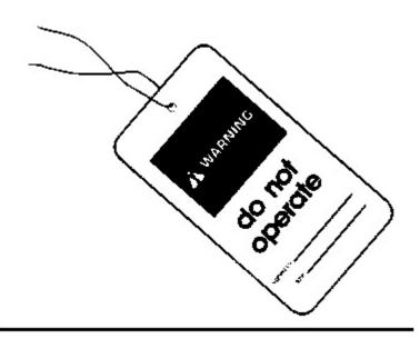
Do not start the engine or move any of the controls if there is a Do Not Operate or similar warning tag attached to the start switch or controls.
