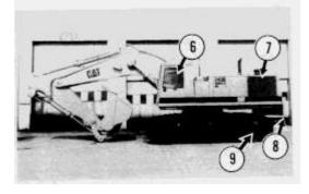
Operator's compartment (6), radiator (7), counterweight (8), and final drives (9).
