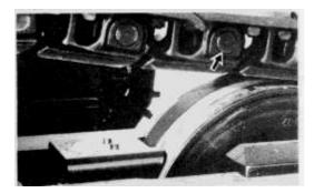
The pins and bushings in a dry track pin joint can become very hot. It is possible to burn the fingers if there is more than brief contact with these components.
