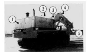
Engine (1), hydraulic tank (2), fuel tank (3), boom (4) and stick (5).
