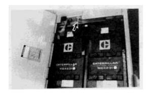
**Disconnect Switch ON** - Insert the key, and turn it to the right, to turn on the electrical system. The switch must be on before starting the engine.
