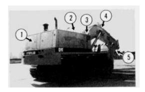
Engine (1), hydraulic tank (2), fuel tank (3), boom (4) and stick (5).
