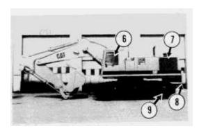
Operator's compartment (6), radiator (7), counterweight (8), and final drives (9).
