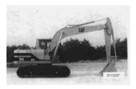
This machine is equipped with a 3054 direct injection turbocharged engine and other specifically developed systems and components such as electronic power unit control system, work mode choice system, two-speed travel motor, etc. The machine is designed primarily for excavating and loading material.
