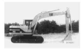
This machine is equipped with a 3064 direct injection turbocharged engine and other specifically developed systems and components such as electronic power unit control system, work mode choice system, two-speed travel motor, etc. The machine is designed primarily for excavating and loading material.
