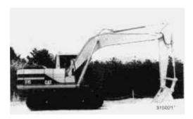
This machine is equipped with a 3054 direct injection turbocharged engine and other specifically developed systems and components such as electronic power unit control system, work mode
