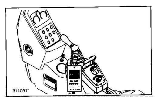
Attach a DO NOT OPERATE, SEHS7332, or similar warning tag to start switch or controls before servicing or repairing the machine. This tag is available from your Caterpillar dealer.
